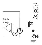
Fig.17 CS pin filter
