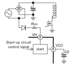
Fig.32 VH pin circuit (2)
