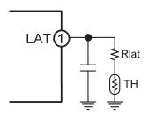
Fig.12 Over temperature circuit
