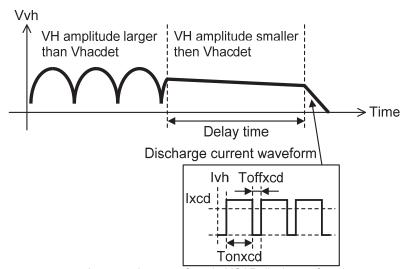
An operating waveform in XCAP discharge function.
