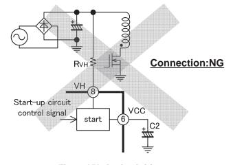
Fig.33 VH pin circuit (3)
