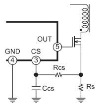
Fig.18 CS pin filter
