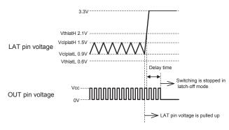
Larch-off operation by pulling up LAT pin voltage
