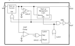
Fig.29 Over voltage circuit block
