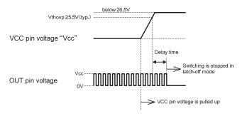
Latch-off operation by pulling up VCC pin voltage
