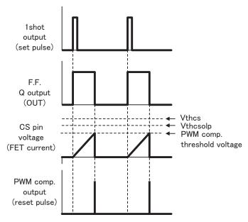
Fig2. Current mode basic operation timing chart
