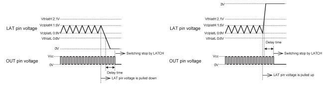
Fig.7 Pull down latch operation
