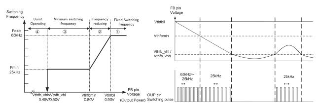
Fig4. Switching frequency – FB voltage (Output power)
