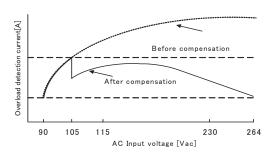
Fig.20Overload detection level on input voltage (2)
