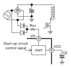
Fig.31 VH pin circuit (1)
