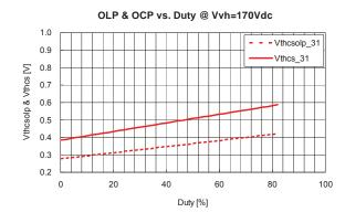
Fig.21 OLP,OCP CS threshold voltage vs. Duty
