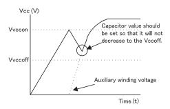
Fig.26 VCC pin voltage at start-up
