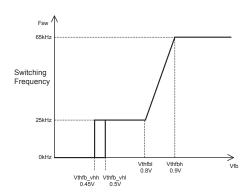
Switching Frequency vs. FB pin voltage
