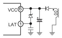
Fig.14 Over voltage circuit (1)
