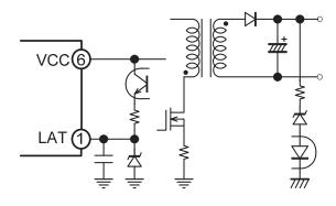
Fig.15 Over voltage circuit (2)
