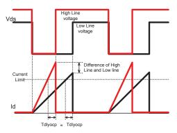
Fig.19 Overload detection level on input voltage (1)
