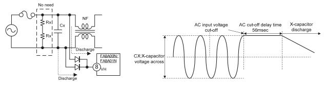
Fig10. VH pin discharge circuit
