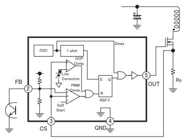
Fig1. Current mode basic operation circuit block
