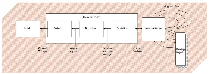
Figure 1 Measurement chain
