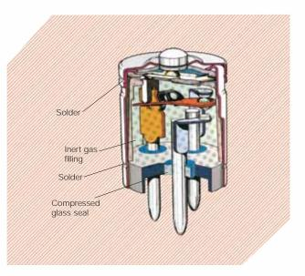
This is the basic component for our whole range of standard 1-pole and 2-poles hermetically-sealed limit switches plus the 3-poles version (special Limit Switches).
