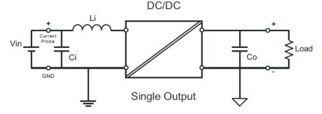
Recommended Output Capacitor to reduce the converter's ripple and noises for single output models is 4.7µF to 100µF and for dual output models is 4.7µF to 68µF connected to both outputs.
