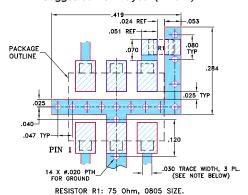
NOTES: 1. TRACE WIDTH IS SHOWN FOR ROGERS ROA350B WITH DIELECTRIC THICKNESS .030" ± .002"; COPPER: 1/2 OZ. EACH SIDE. FOR OTHER MATERIALS TRACE WIDTH MAY NEED TO BE MODIFIED. 2. BOTTOM SIDE OF THE PCB IS CONTINUOUS GROUND PLANE.
