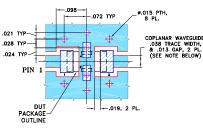
NOTES: 1. COPLANAR WAVEGUIDE PARAMETERS ARE SHOWN FOR ROGERS RO4350B WITH THICKNESS .020" ± .0015".
