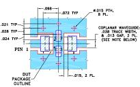
COPLANAR WAYEGUIDE PARAMETERS ARE SHOWN FOR ROGERS RO4350B WITH THICKNESS .020" ± .0015". COPPER: 1/2 OZ. EACH SIDE. FOR OTHER MATERIALS TRACE WIDTH & GAP MAY NEED TO BE MODIFIED.
