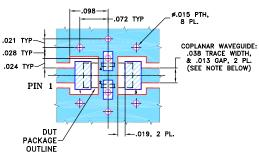
NOTES: 1. COPLANAR WAYEGUIDE PARAMETERS ARE SHOWN FOR ROGERS RO4350B WITH THICKNESS .020" ± .0015".
